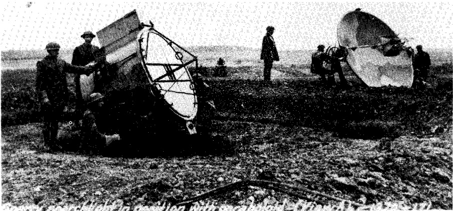
American paraboloid and searchlight in position to track and illuminate attacking enemy aircraft.
